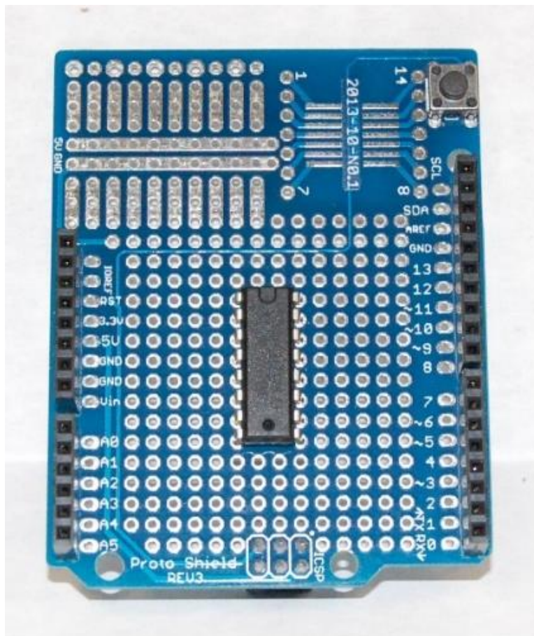
Figure 1: Placement of Motor Driver on Protoboard.
