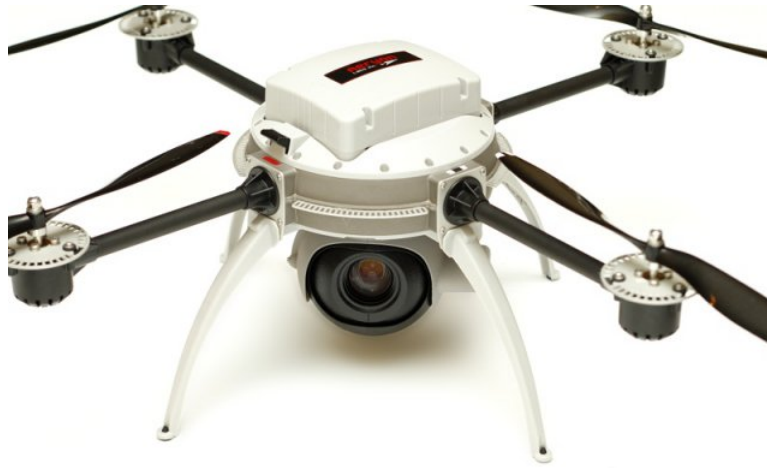
Figure 13: Aeryon Scout for structural inspection. It also has thermal imaging capabilities. [13]
